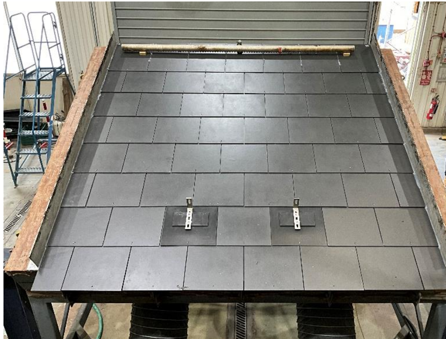
Figure 2: Specimen 2 on the BRE test rig.
