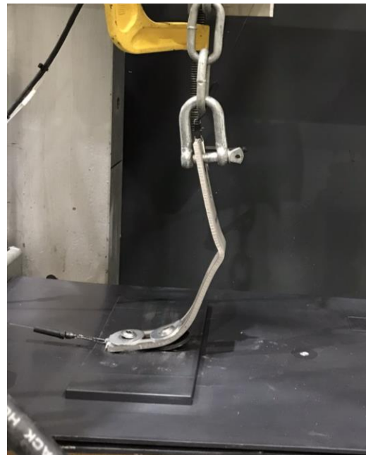
Figure 5: Photo SF1 during the test, the hook had significantly deformed.
