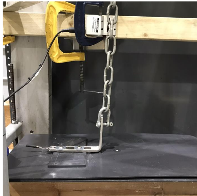
Figure 2: Specimen 2 on the BRE test rig.
