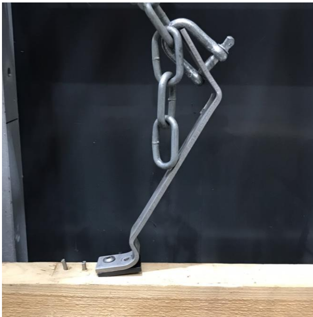
Figure 4: Photo PF1 during the test. The hook had significantly deformed, and the screw head of one screws had broken off.
